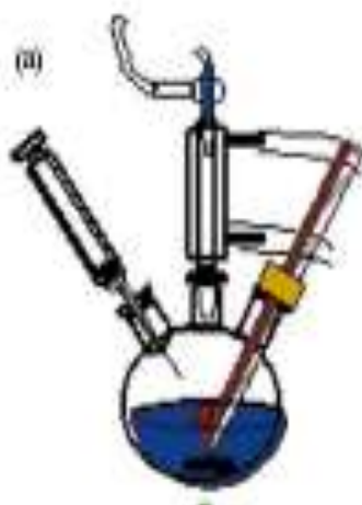
Fig.3.1: Setup for synthesis PbSe NC colloidal solutions. Taken from C. B. Murray et al. 53 )
