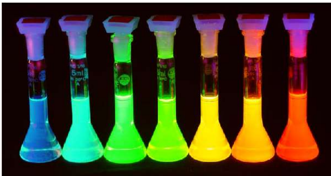
Fig. 1.1: The image above represents the fluorescent-emission colors of cadmium selenide nanocrystals, or "quantum dots," excited with a near-ultraviolet lamp 3
